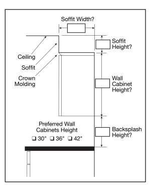
CREATE ELEVATION DRAWINGS - Now, draw an elevation of each wall and locate all openings. Be sure to include the ceiling height and show soffits (boxed build-down from ceiling), if you have them or plan on adding them. For easy identification, use the symbols shown below to locate water lines, drain lines, electrical outlets/switches, etc.
